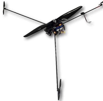
comprises a triangular quadrotor with a single large main rotor for high efficiency, and three small rotors for control and counter-torque. The Y4 has an approximately 200% improvement in energy efficiency over existing state-of-the-art systems. It can perform any task done by a conventional quadrotor or remote helicopter; however, it has superior flight times and remarkable hovering stability, positioning it for many commercial/industrial applications.
